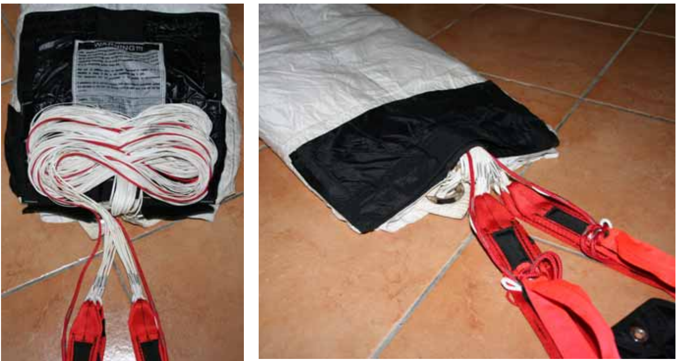
Figure 7a & 7b: S-fold lines into Tail Pocket
